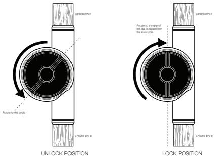
The Basil Hinge should feel easy to lock and unlock. If jammed, do not force the hinge to close as it may cause damage.
